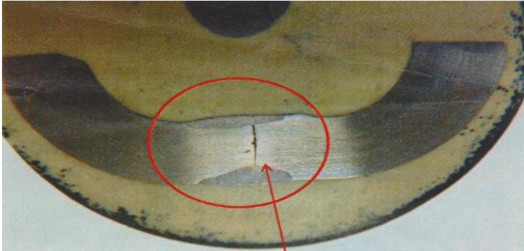
**Figure A3 Showing a welding penetration defect of a chain link due to inadequate manufacturing processes.**
