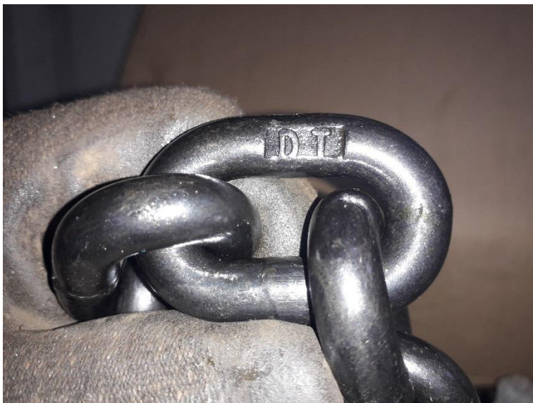
Image 2 – Factory Identifier D and Grade T marked chain
