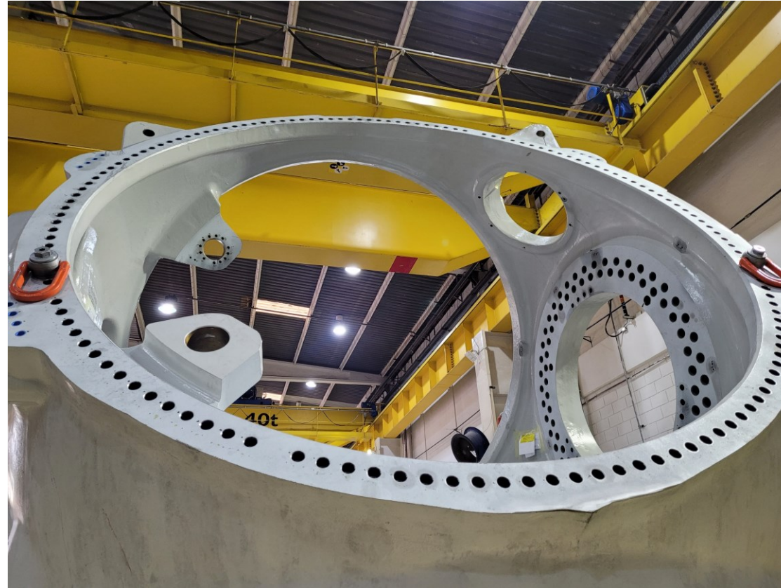
lifting points for handling hubs through production process
