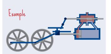
A steam engine uses pneumatics to move forward. Imagine a double acting cylinder with a wheel attached. As the cylinder is pushed out, the rod moves to the left, and as the cylinder is pulled in, the rod moves to the right. The movement of the rod then rotates the wheel, and this is how the steam engine moves.
