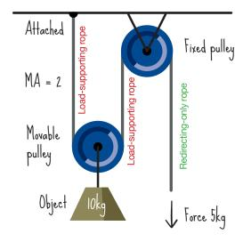
The factor by which the force decreases if known as the Mechanical Advantage (ME). We can work out the ME by dividing the weight of the load by the force required to lift it. For a pulley that halves the force required, the ME is 2. For a pulley that thirds it, it is 3.
