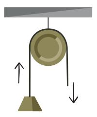
A simple pulley consists of a rope attached to a wheel. The wheel has dents where the rope fits in.
